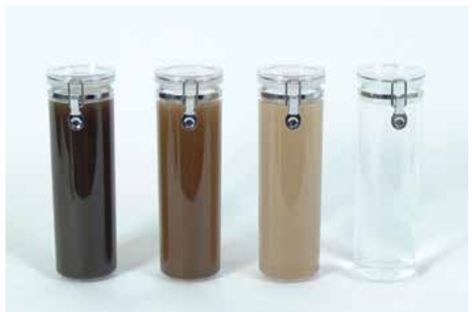
Water samples from system treated with EnwaMatic® technology. From day 0 to day 30 to the right.
